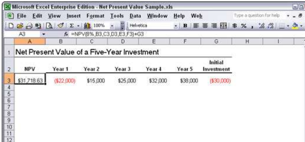
Figure 2: Using the NPV function to calculate the net present value of an investment.
